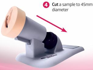
**Place** the sample onto the spiked specimen holder
