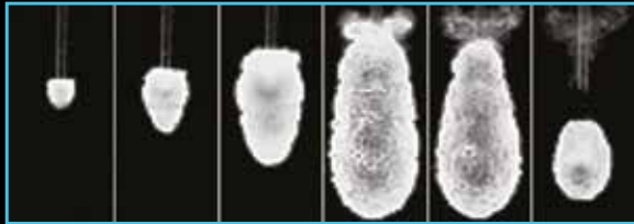
Bubble Dynamics of Vapor Tunnel™
