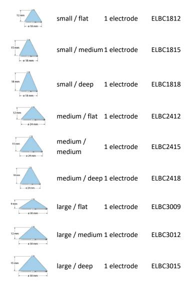
CAUTION! The BIO-CONE electrodes require a handpiece with a shaft diameter of 2.4 mm (3/32"). Handpieces for the ErondSURGcan be find in category 9. Conization can be performed only with high frequency units offering a frequency of at least 400 KHz. The higher the frequency the smoother the probe can be extracted.
